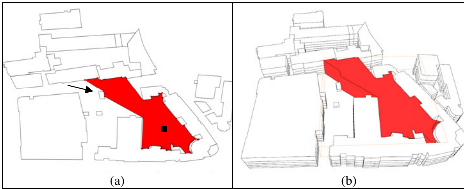
Fig. 3. (a) 2D Isovist view (b) Extruded 2.5D Isovist in a 3D environment
