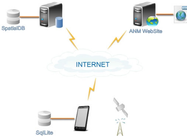
Fig. 1. The GIS system architecture. A mobile database (SqlLite), a spatial database (GeoServer) and a web-service.
