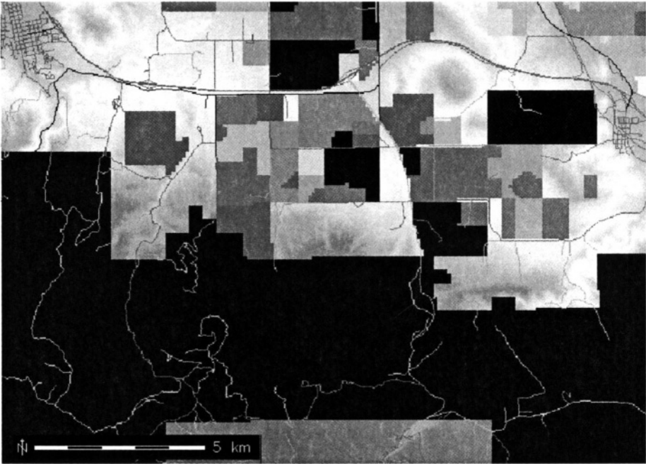
Figure 5.4. Map composite of roads, land use map and elevation model created with r.patch (Spearfish area)
